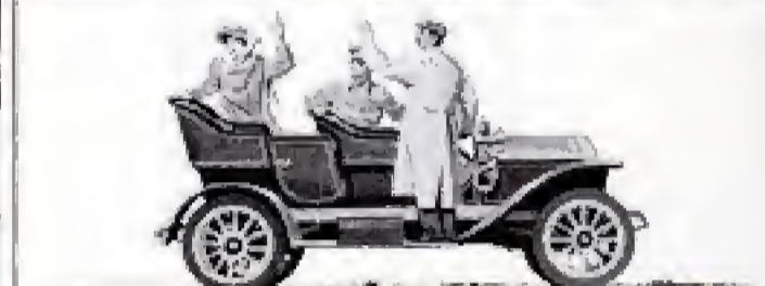
1907 KNOX WATERLESS was advertised as the "car that obviates the tow." The makers claimed that their air-cooled engine never overheated, thanks to hundreds of pins screwed into the cylinder walls to carry off engine heat.
